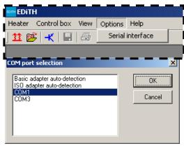
\*Note: If you receive this message, either you selected the incorrect com port or the USB to serial adapter has been configured improperly.
